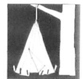
Parachute material can be used to make a tepee, but even simpler is to suspend one from a tree. Use the sides for a windbreak and keep the fabric as waterproof as possible. For the best shelter, use the bottom edge of the parachute to make a windbreak and make it airtight by taping it.
